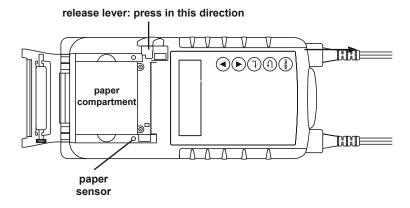
2. Place a new roll of paper in the compartment, and pull the paper forward so that it extends past the serrated edge of the paper slot.
